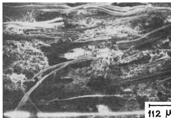
Fig. 29. SEM photomicrograph of the tear fracture surface of blend 30B 7 ; well-ordered bundles of fibers placed across the surface.
